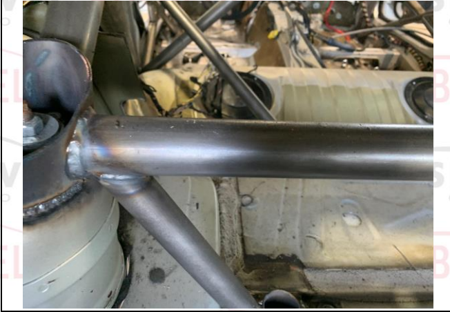
PHOTO 12 SHOULDER HARNESS ATTACHMENT - DRIVER
