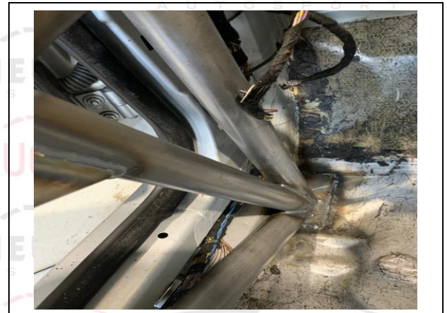
PHOTO 6 FRONT ROLLBAR TO FLOOR ATTACHMENT
