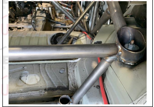
PHOTO 13 SHOULDER HARNESS ATTACHMENT - CO DRIVER
